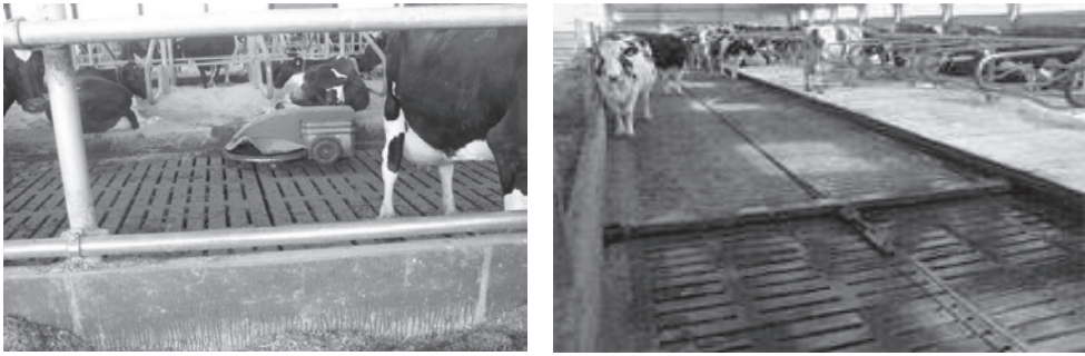
Figure 1. Two methods for scraping slatted floors in dairy houses: a robotic scraper (left) and a wire-propelled scraper (right).
