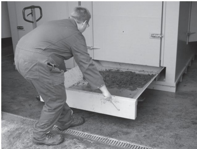
Figure 1. The removable manure tray enables rapid collection and cleaning of manure.
