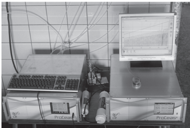
Figure 2. Measuring device: multi sampler (left) gas analyser (right).
