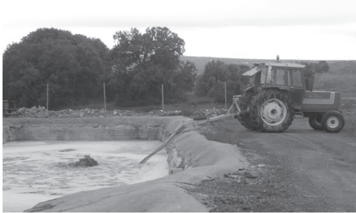
Figure 1. Aeration treatment on pig slurry storage.
