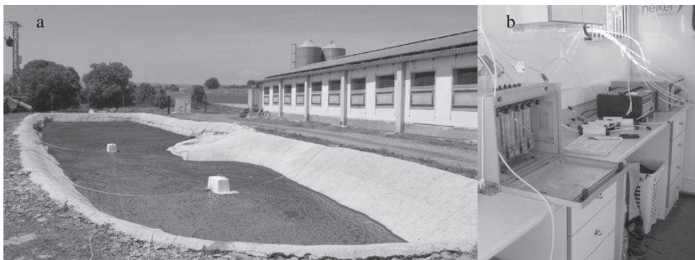
Figure 2. (a) dynamic chamber gas sampling system and (b) in situ gas monitoring unit.
